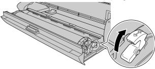
**9** Pull up the leading edge of the roll media, and then from above pass the sheet past the paper guide as shown in the illustration.
